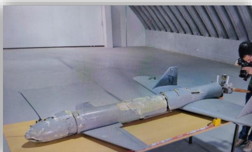
Damage to the aircraft and the attacking UAV model (courtesy of Tal Inbar/ "Mosaic"- Technical Intelligence Brief)
