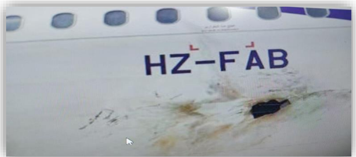
Damage to the aircraft and the attacking UAV model (courtesy of Tal Inbar/ "Mosaic"- Technical Intelligence Brief)
